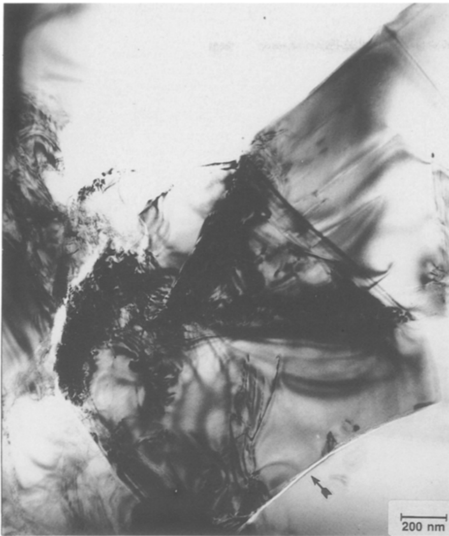
Figure 18 Intergranular crack (marked with arrow) and dislocations in alumina impacted at 4.6 GPa in aluminium capsule (compression + tension).
