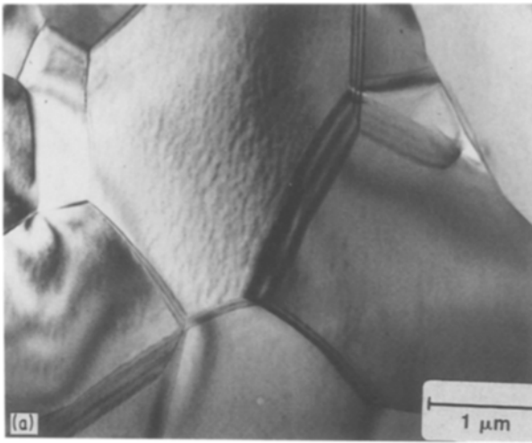
Figure 16 Transmission electron micrograph of as-received HP-alumina ( 4\ \mu\text{m} grain size): (a) general grain morphology; (b) hexagonal-shaped void.
